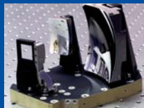
The three mirrors anastigmat telescope from the GERB experience (METEOSAT). Its weight: 1kg650, its dimensions: 17cm x 13cm.
