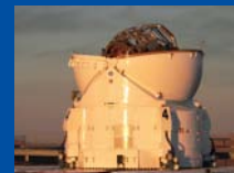
The mobile ATS (Auxiliary Telescope System) designed and manufactured for ESO VLT. Its characteristics are: 32 T, 6 m high and a primary mirror of 2m.
