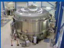
XMM space simulator delivered to Liege Space Centre (CSL), whose dimensions are 7 m high and 6.5 m in diameter.
