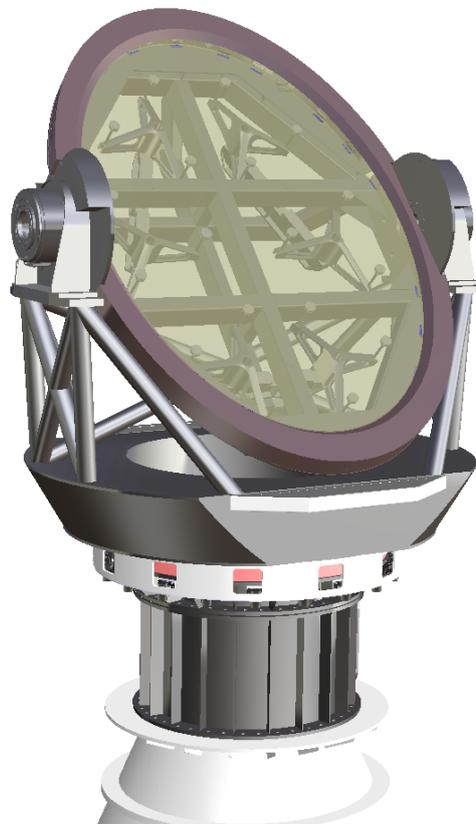
M3 Support System and Positioner Assembly (M3SSPA)
