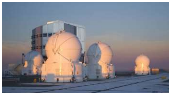
ATS (Auxiliary Telescope Systems), “mobile” telescopes in the VLTi in Chile (Cerro Paranal)
