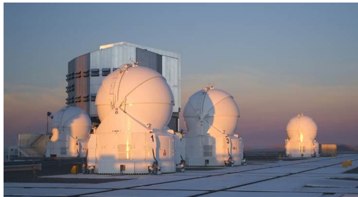
ATS (Auxiliary Telescope Systems), “mobile” telescopes of the VLTi in Chile (Cerro Paranal)
