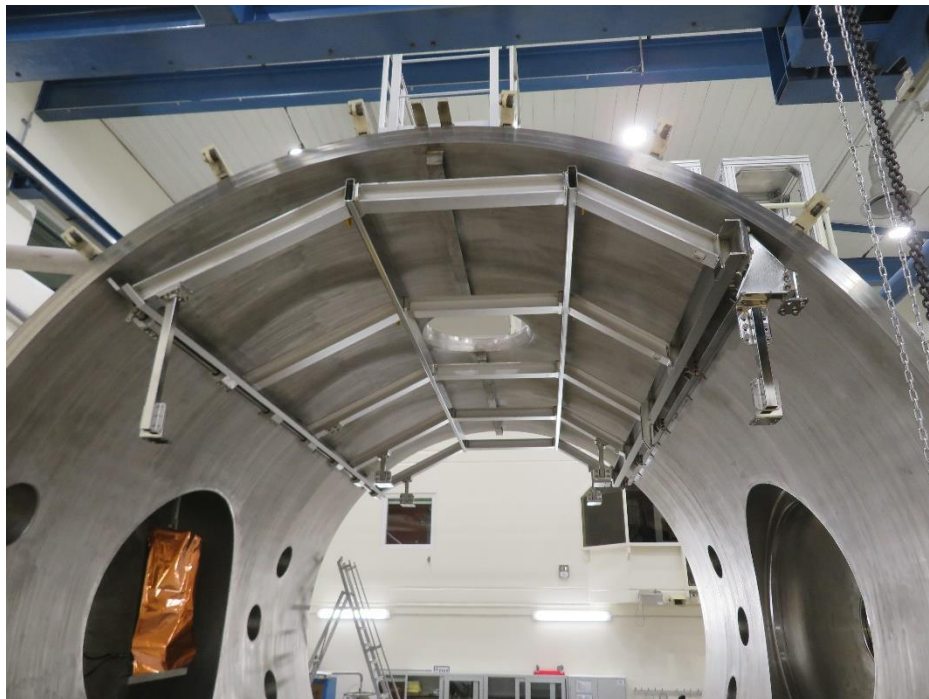
Lift truck structure integrated in Focal 5 vessel
